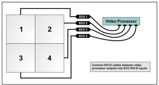
When adding a video processor, connect the Ethernet connection to the master ECU. Multiple video processors might be required if multiple connections are required. For example, a Vista Spyder has eight connections; an additional video processor is required if you are using more than eight ECUs.
