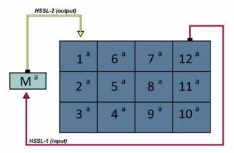
By default, the media source connected to the master ECU will be scaled over the entire array.
