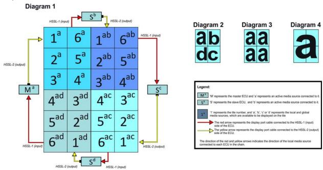
By default, the media source connected to the master ECU is scaled over the entire array.
