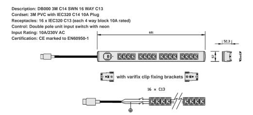
The PDU should have local safety/regulatory approvals and adequate electrical current capabilities.
