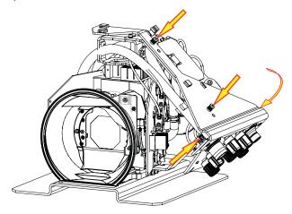
5. Install zip ties to secure the hoses and mini SAS harnesses to the shipping bracket.
