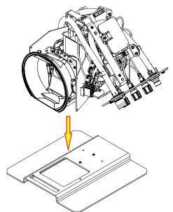
2. Install the three screws to secure the light engine to the shipping base plate.
