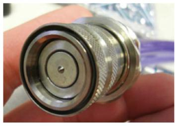
As the female ring releases and moves to its closed position under spring load, it can cause some coolant to be ejected.
