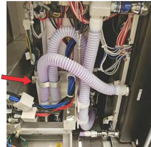
6. Place cloth wipes around the cooling hose connection points to capture any excess coolant that may drip upon disconnect.
